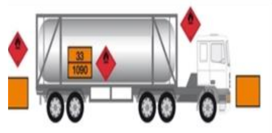
Transport units with individual tank divisions
