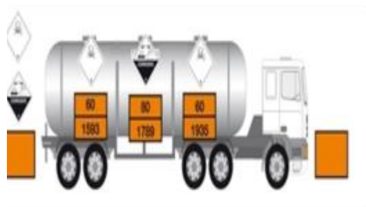
Transport units with multiple tank divisions
