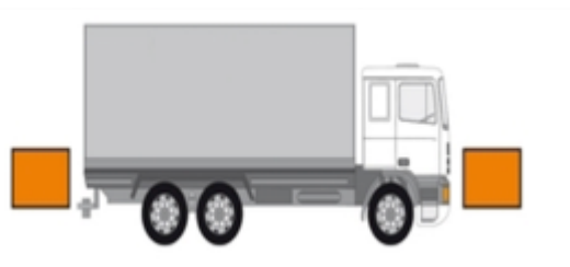
Packaged Dangerous Goods
